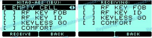
Press OPEN or CLOSE on keyfob. After the signal is successfully received you will see [+] in RF KEY FOB and RF KEY ID
