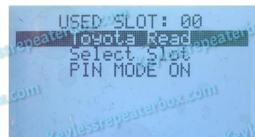
Depending on the selected PIN mode code the device will turn on either locked or unlocked. To change the PIN code mode, you must select the menu item **PIN MODE ON (OFF)**. In this case, the state of the mode will change to the opposite. Menu item
